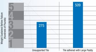
Tested in accordance with ASTM C 1492-03 and performed with low profile, lightweight tile.
