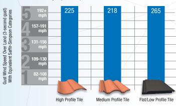
ASCE 7-10 Wind Design Standard. Exposure C, 30 foot mean roof height, Importance factor 1.00, High Profile based on a tile factor of 1.407, 2:12 to 6:12 slope, gable/hip roofs.
