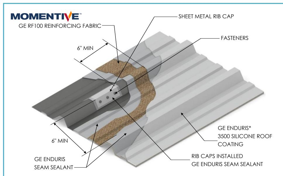
NOTE: RIB CAPS ARE REQUIRED OVER BROKEN RIBS; AFTER INSTALLATION, SEAL THE RIB CAP PERIMETER AND FASTENERS WITH ENDURIS SEAM SEALANT
